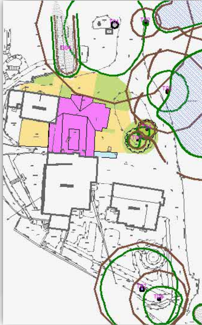
Figure 4: Proposed Site Plan, Drawing No. 22.425 S02.05 (Swain Architecture) with Tree Constraints Plan, Drawing No. Arbtech TCP 01 (Arbtech) overlaid showing no RPA incursions.
