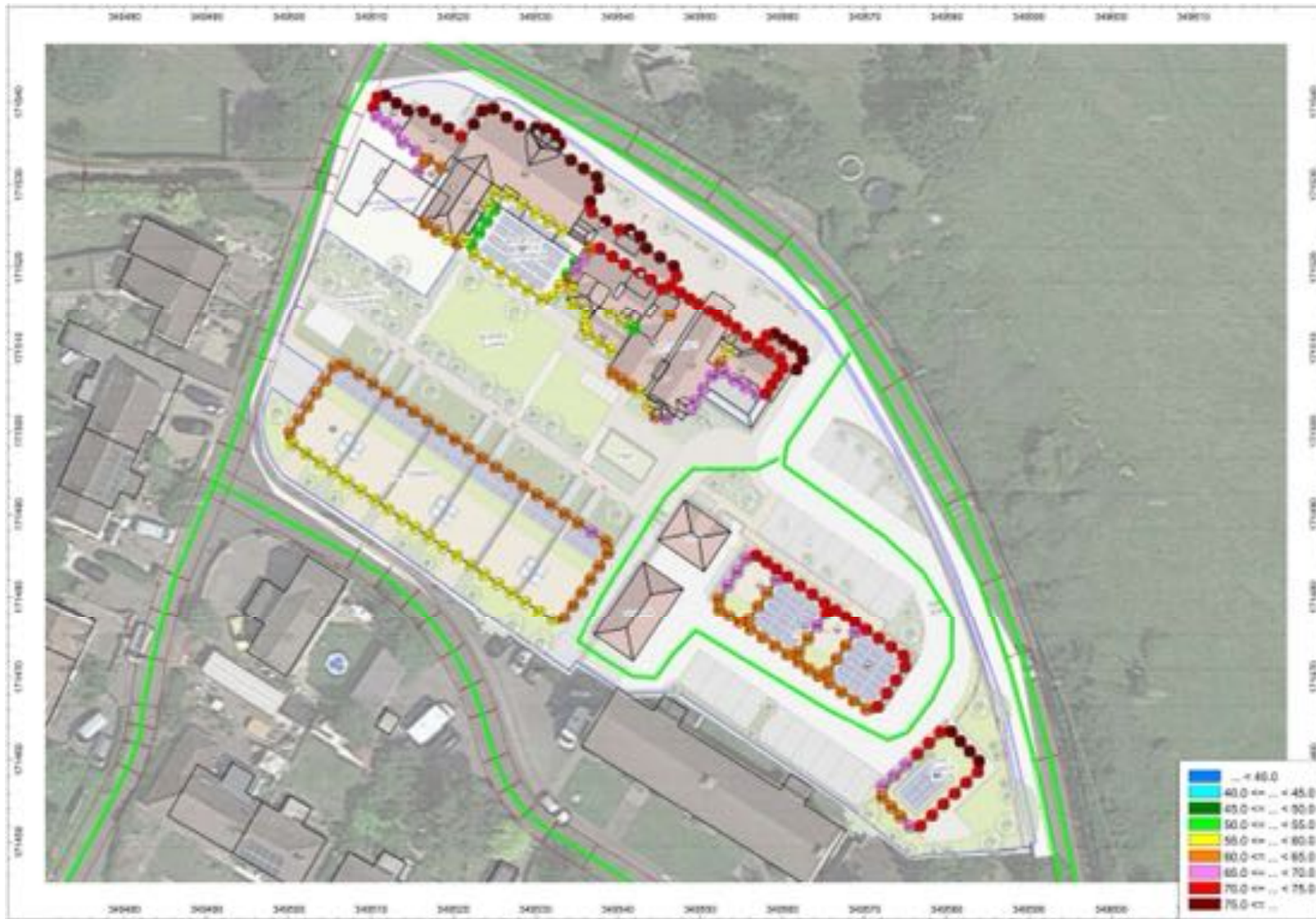
Figure D.9 – Proposed development - Predicted façade 10 th highest dB L AFmax exposure levels – Night-time (23:00 – 07:00)
