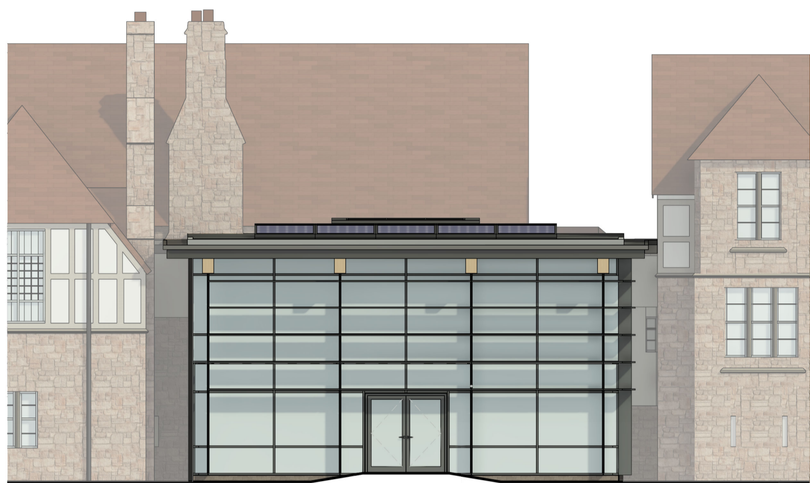
3 Office Extension - South Elevation SCALE 1 : 100
