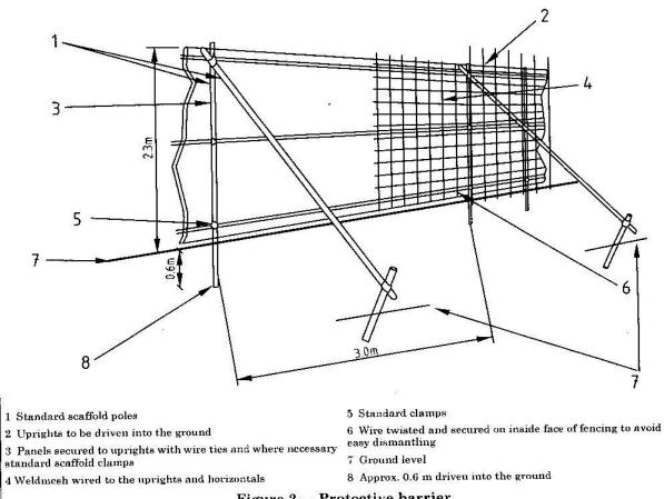
Figure 2 — Protective barrier
