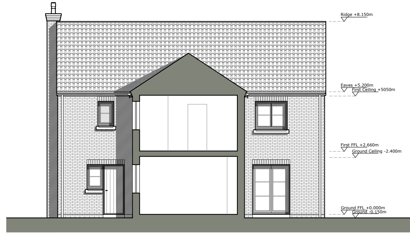
04 PROPOSED SECTION THRU DAYROOM/BEDROOM 1 1:100
