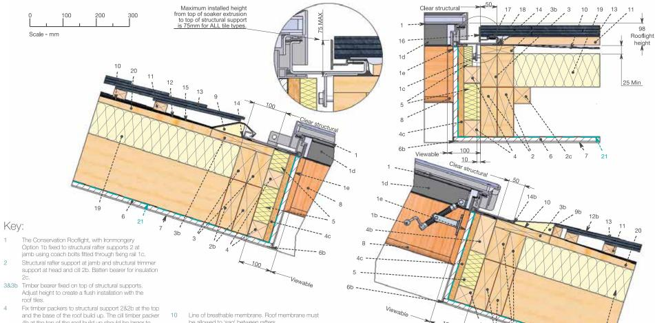
4b at the top of the roof build up should be larger to provide a secure fixing point for the ironmongery. Fix 18mm ply packer to the timber packers.
