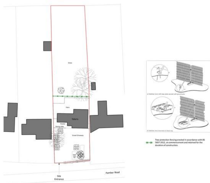
Image 09: Tree protection fencing indicated to prevent contractor encroachment.
