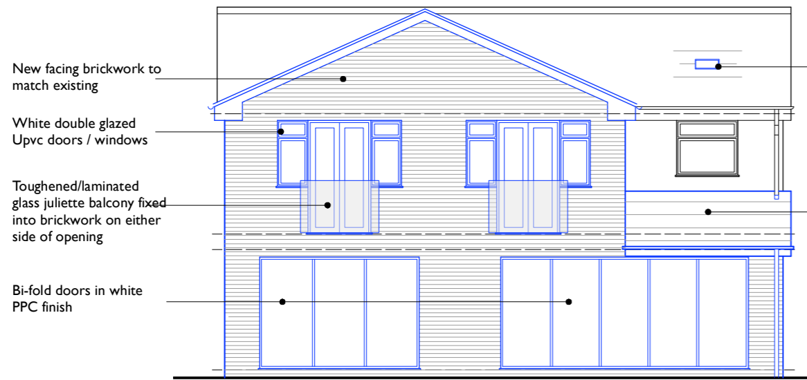
REAR (EAST) ELEVATION AS PROPOSED
