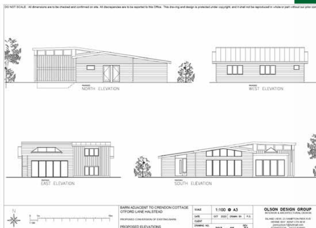
Figure 4: Proposed Conversion of the Existing Barn
