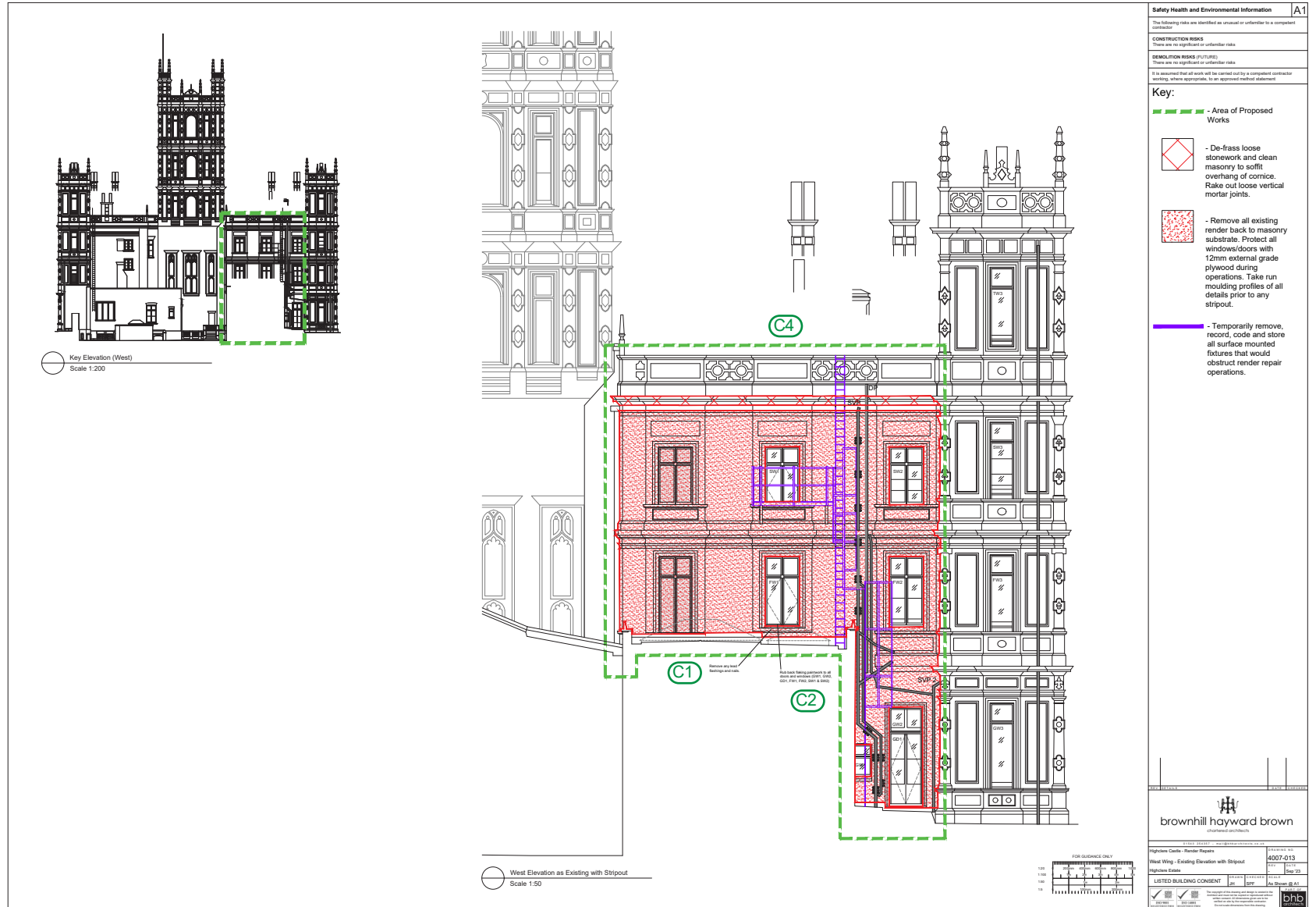
Fig.18 (Below) Architect's drawing showing the areas of render removal to the Castle's West Elevation.
