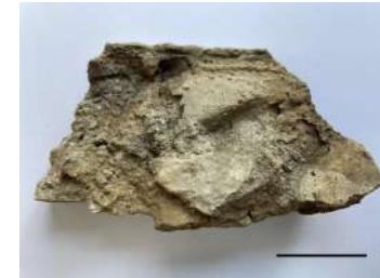
Plate 2. Image showing the underside of the sample as received. The sample shows signs of leaching and binder dissolution. Scale bar = 20mm.
