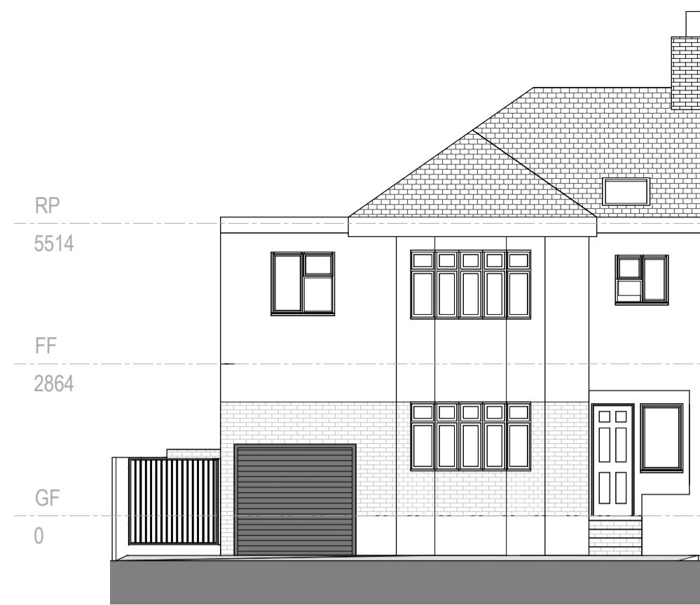
Front Elevation - Existing 1:100
