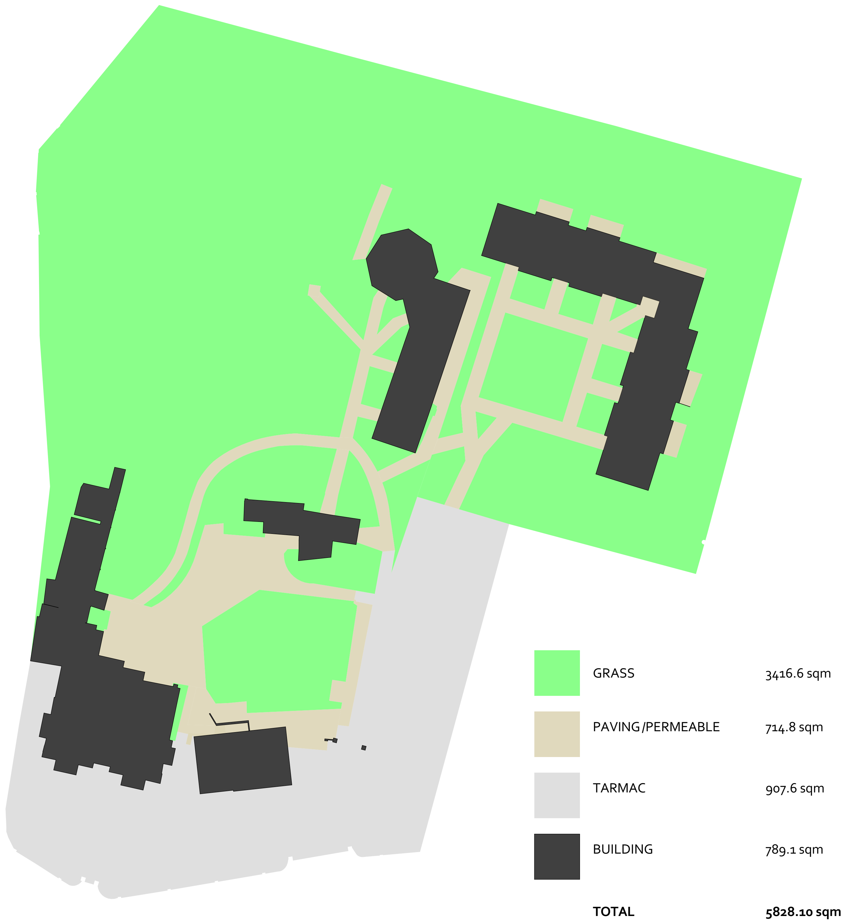
Site Wide Surface Materials As Existing
