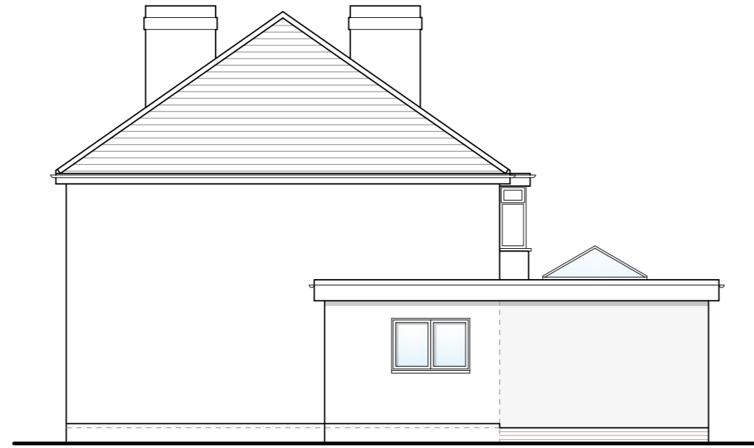
SIDE ELEVATION AS PROPOSED Scale 1:100 Render to match existing dwelling
