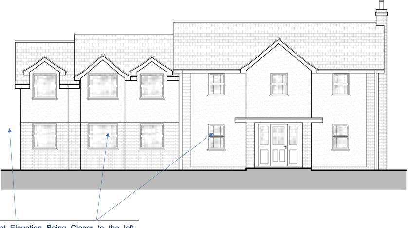
Front Elevation Being Closer to the left boundary, further forward to the front boundary and larger windows
