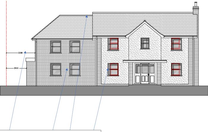
Inset side elevation at first floor level to create 3000mm separation from left side boundary. Reduced number of windows and size. Reduced height of overall building level
