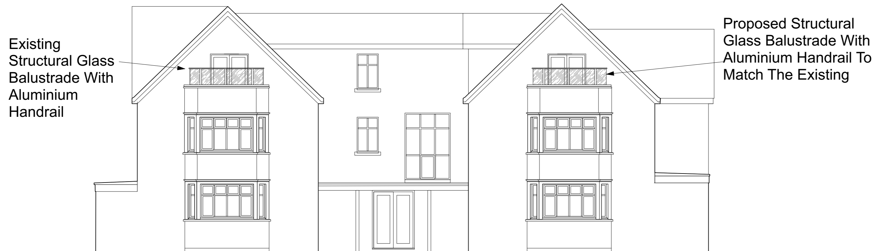
Proposed West Elevation
