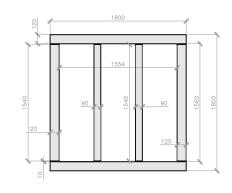
Main window measurements: 3no. Window openings W460 x L1560 Stone Lintel 1800 x H120 x D150 Stone Cill W1800 x H120 x D250 with fall away from window Stone column (side) x2 W120 x H1540 x D150
