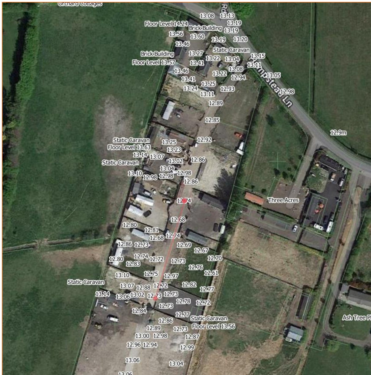
Figure 12: Topographic surveyed overlay on aerial imagery. Red line shows section of site access with a flood depth exceeding 25cm (Source: SJM Surveys Ltd, Google)
