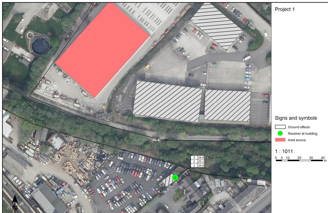
Figure 3 – Sound propagation from waste transfer building to nearest house
