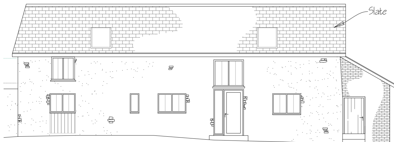
South scale 1:100 Metal Profile Roof Stone, Brick & Rendered Walls Metal, Timber Windows & Doors
