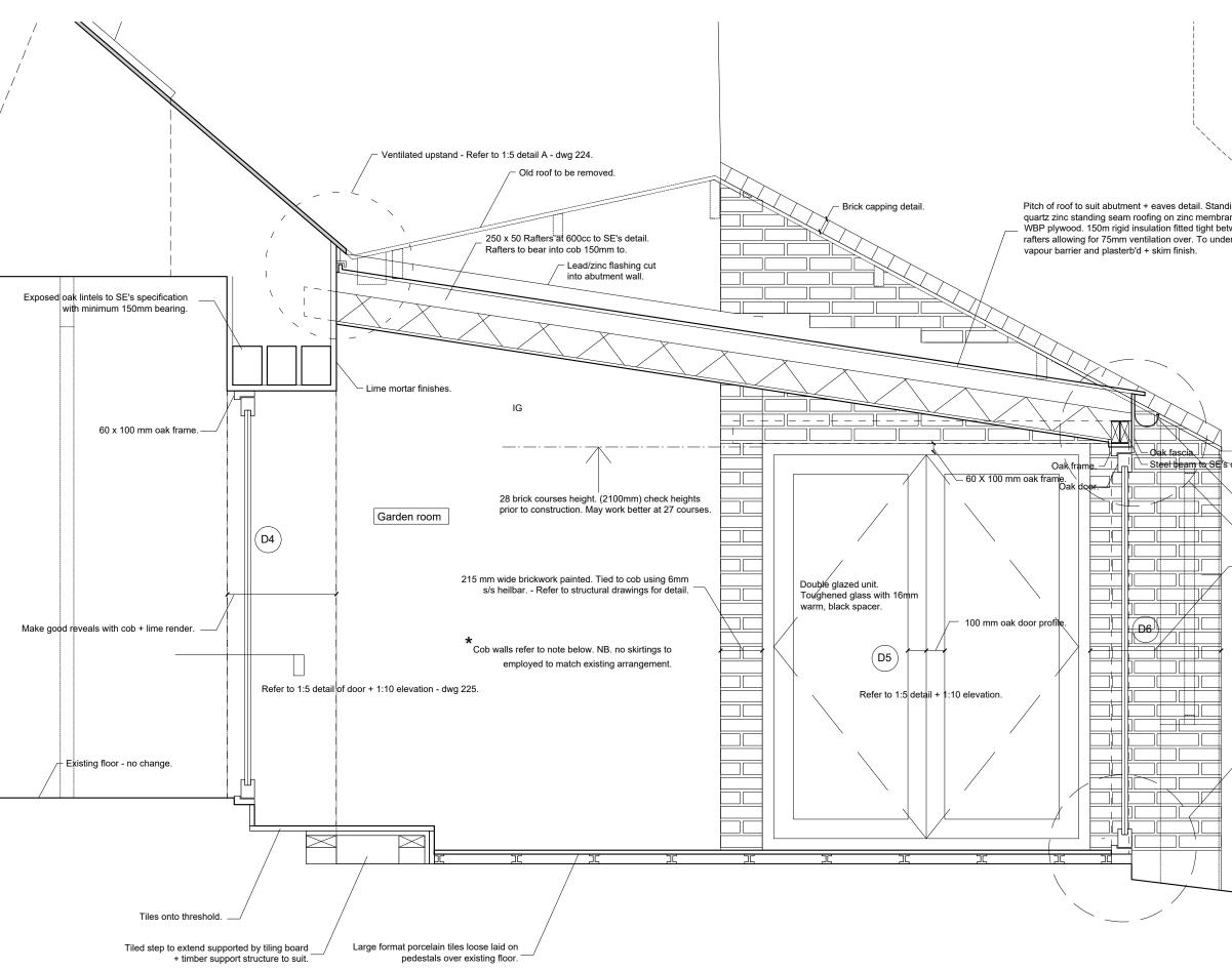
Internal wall treatement: cement plaster to be removed from annex and north walls of house and conservatory area, replace with new lime putty render and breathable paint system. Render by specialist builder. Refer to method statement.
