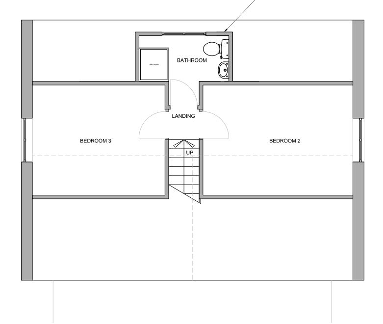
PROPOSED FIRST FLOOR PLAN SCALE 1:50
