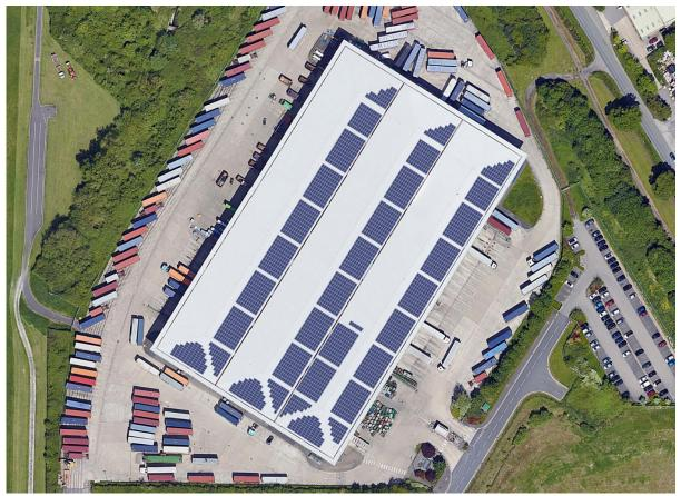
Proposed layout (not to scale). The design allows for 1.5m of space from the roof edges to ensure maintenance and safety regulations are met. Exclusion zones as identified by structural engineers have also been incorporated into the design.
