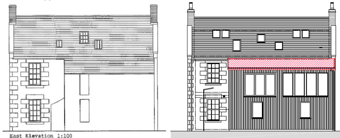
Δ Drawings showing old two storey 'outshot' from previous planning application and existing extension
