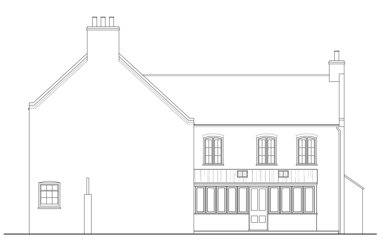
ELEVATION SHOWING POSITION OF NEW CONSERVATION ROOFLIGHTS
