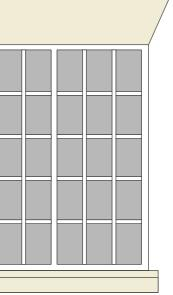
small pane metal window to brickwork extension to main house, 2-part side hung opening window, stone external sill, stone lintel.
