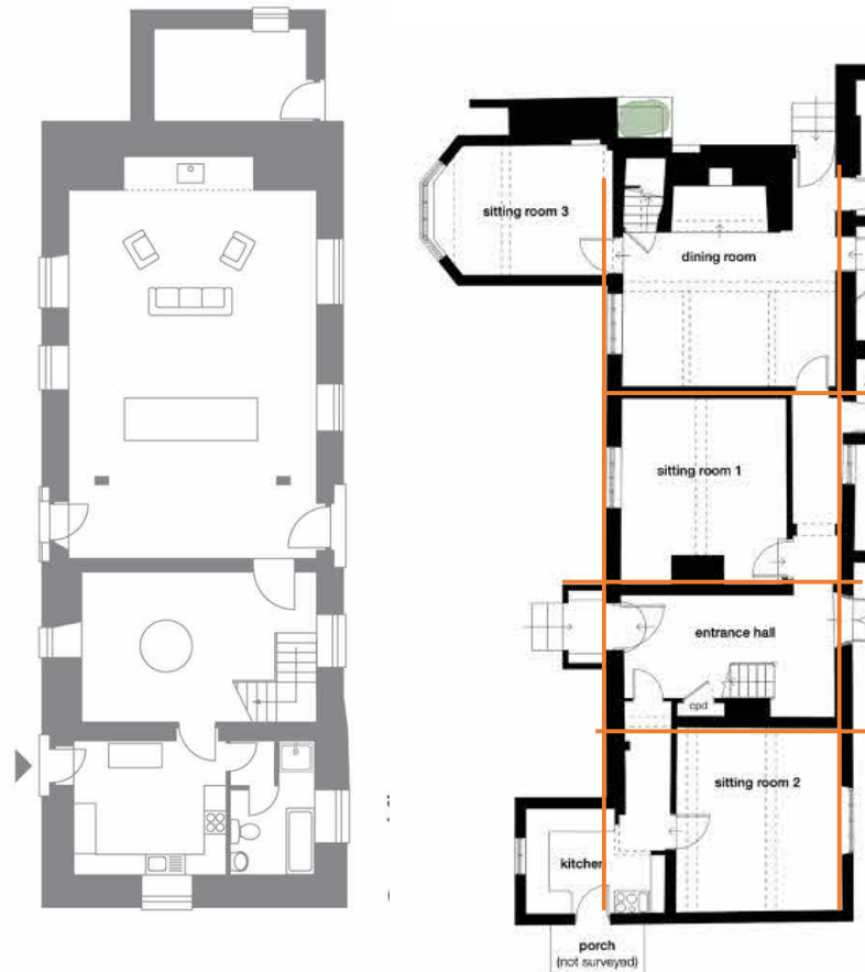
Fig 15. Left: The plan for of Plas Uchaf, near Corwen, Denbighshire, a hall house of c1400; and the ground floor plan of Churton Hall. These are at different scales but the outline in orange of Churton Hall shows the possible layout of the cruck framed hall. Sitting rooms 2 and 3 were added in the 17 th century with a lateral chimney to the east elevation. At this time floors and the stairs would have been inserted.
