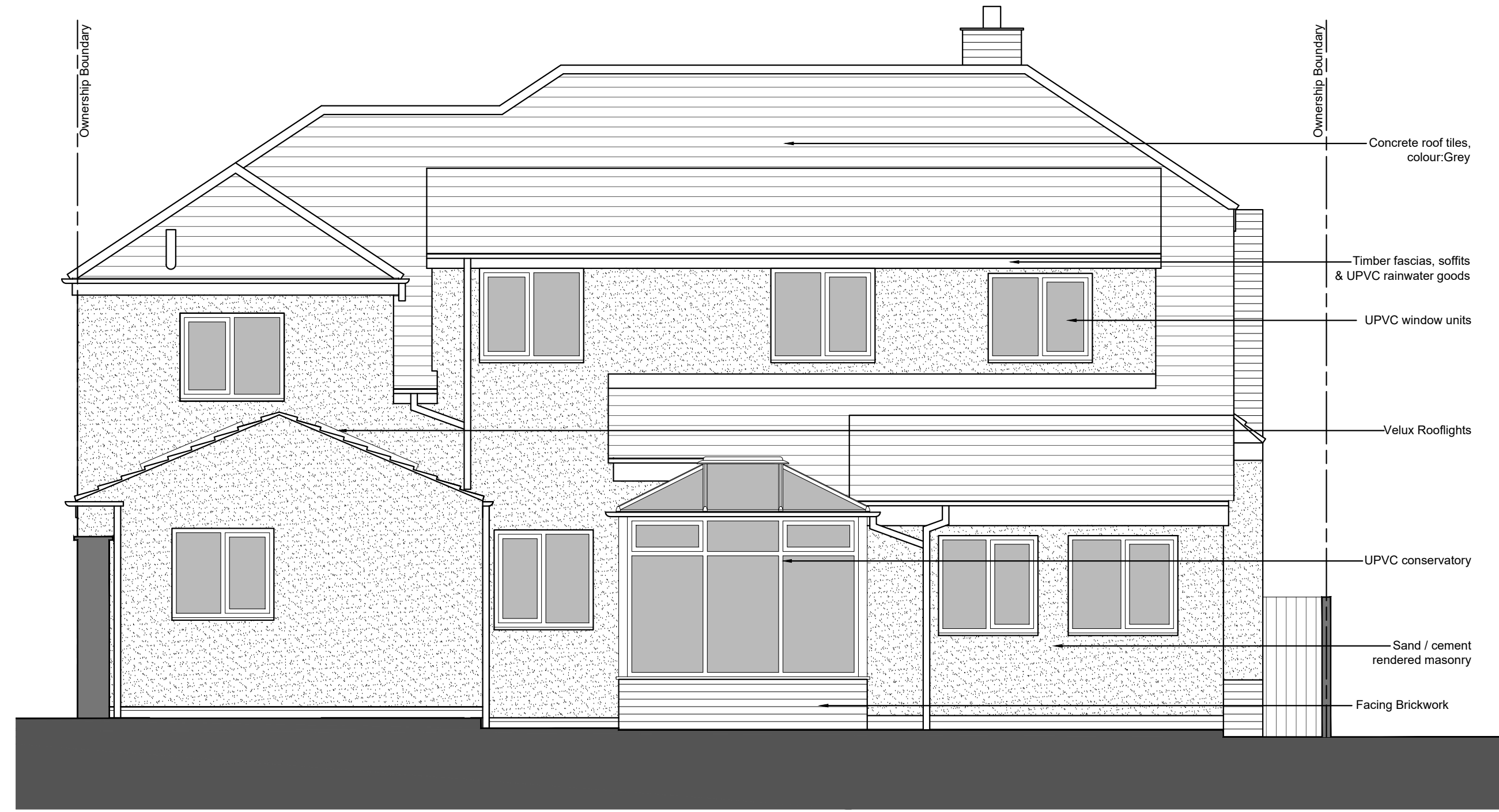
EXISTING REAR (NORTH-EAST) ELEVATION 1:50
