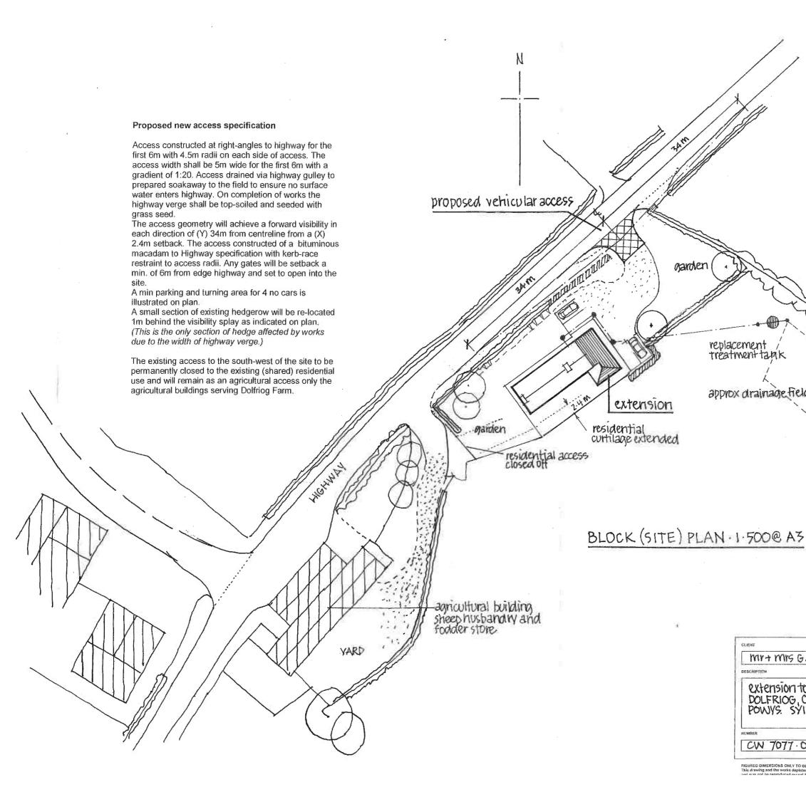
The existing 'septic tank' unit is clearly defective and will be replaced with new underground unit eg Marsh ensign treatment plant 6-8 person to comply with BSEN12566-3:2009 and BS 6297;1983. Installed strictly to site installation guide with separate inflow and outflow IC's prior to connecting to existing drainage field. The drainage field shall be checked by drainage contractor to ensure viable drainage system is available)
