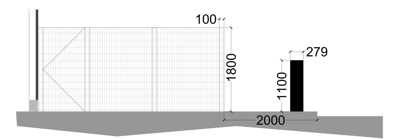
Proposed Fence - Option One: Double palisade fence panel
