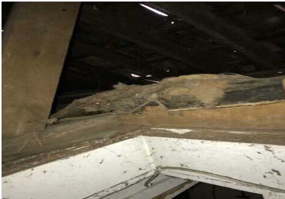
Sample 03 – Thermal insulation – No asbestos detected.
