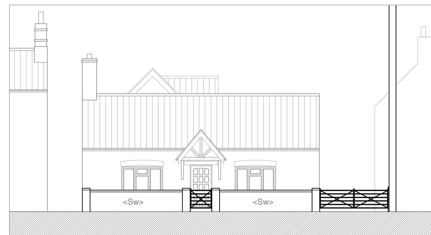
Proposed South-West Elevation 1:100 (neighboring dwellings shown indicatively) <Sw> = Stone boundary wall & cappings
