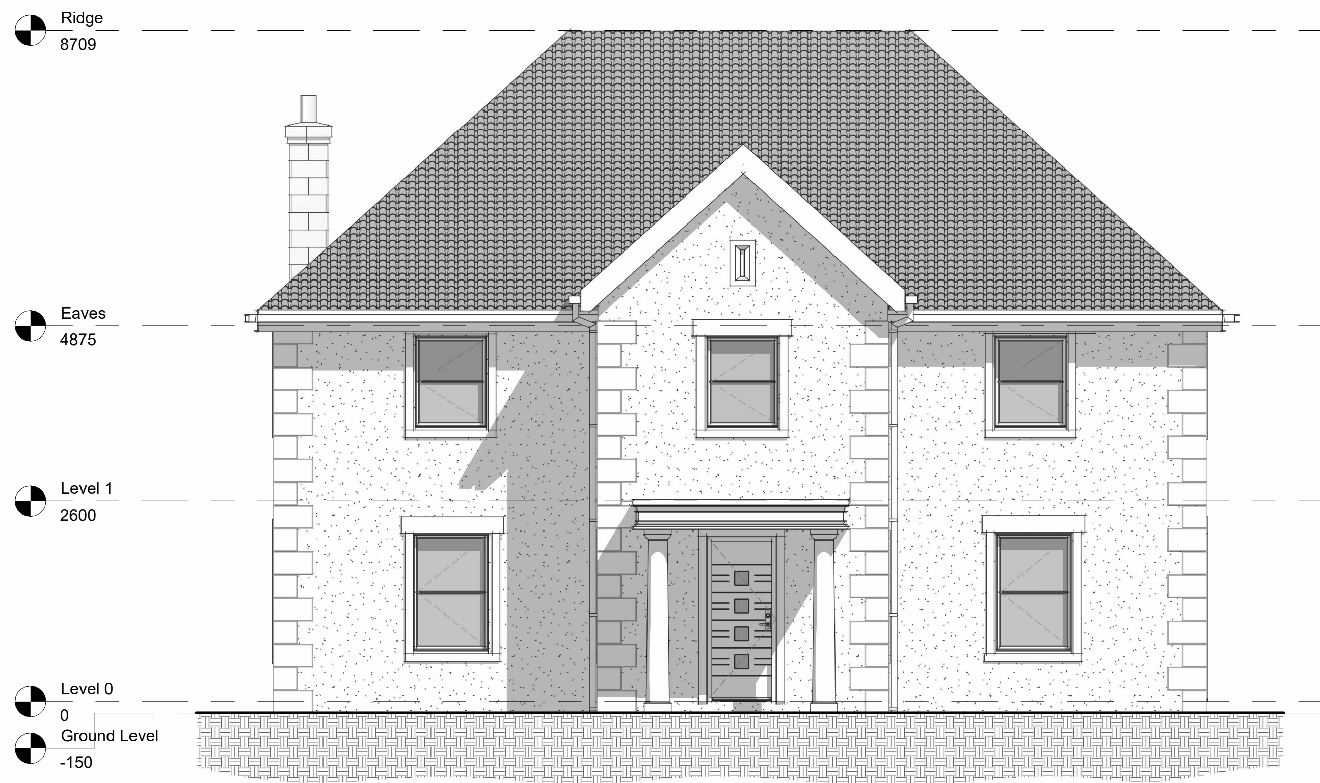
1 DWELLING - NORTH ELEVATION - EXISTING 1 : 50
