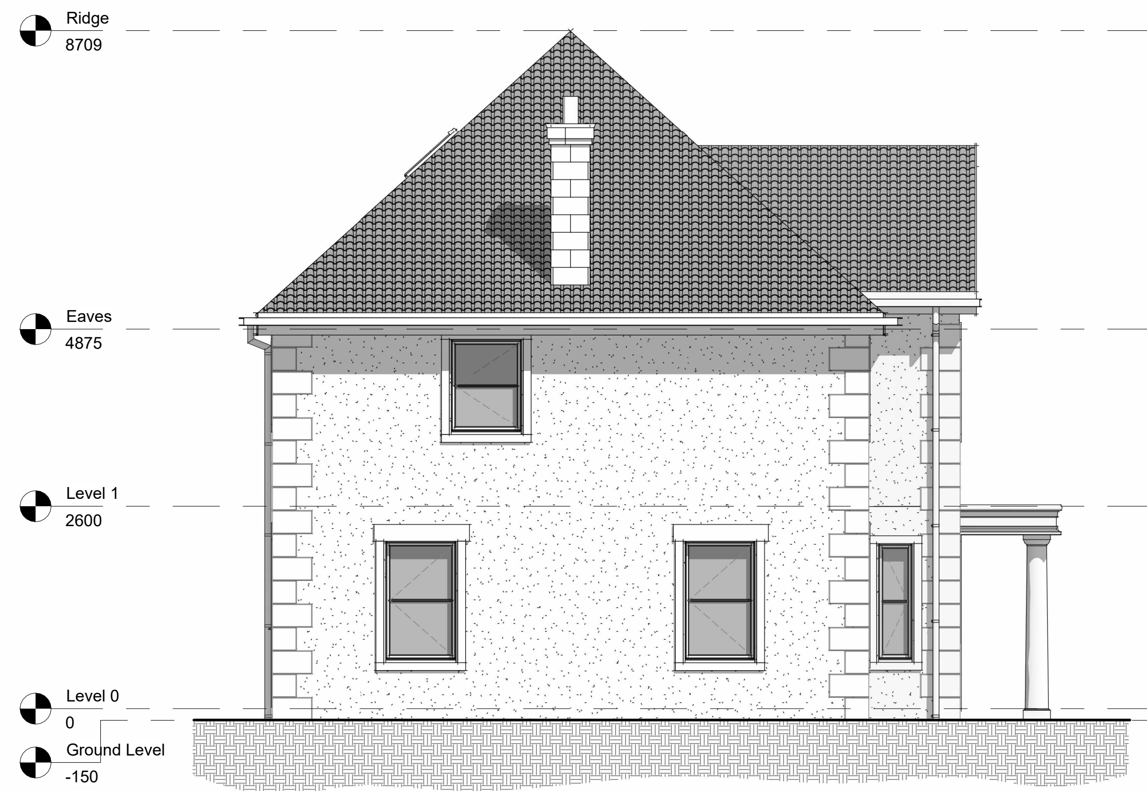
2 DWELLING - EAST ELEVATION - EXISTING 1 : 50
