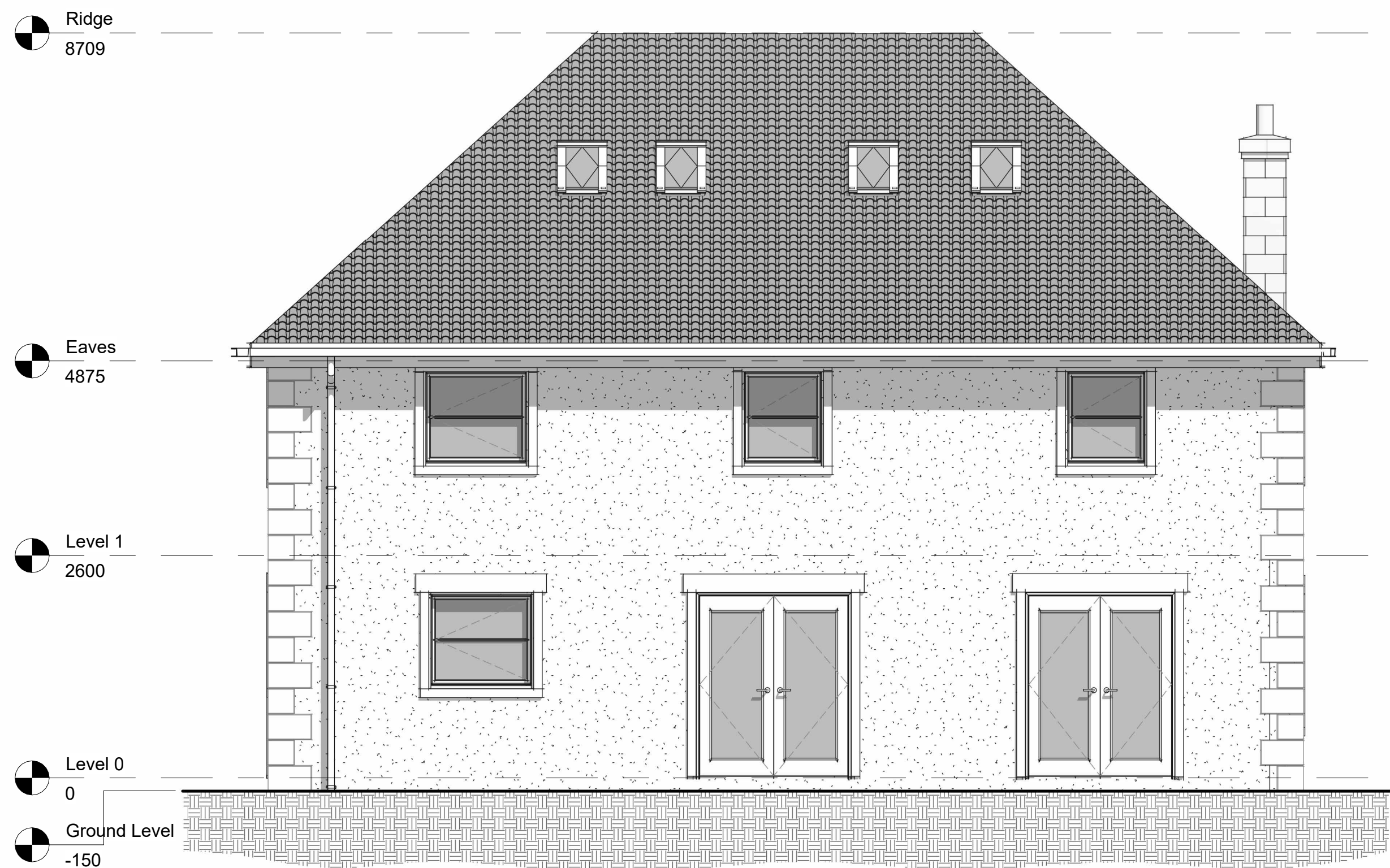
3 DWELLING - SOUTH ELEVATION - EXISTING 1 : 50
