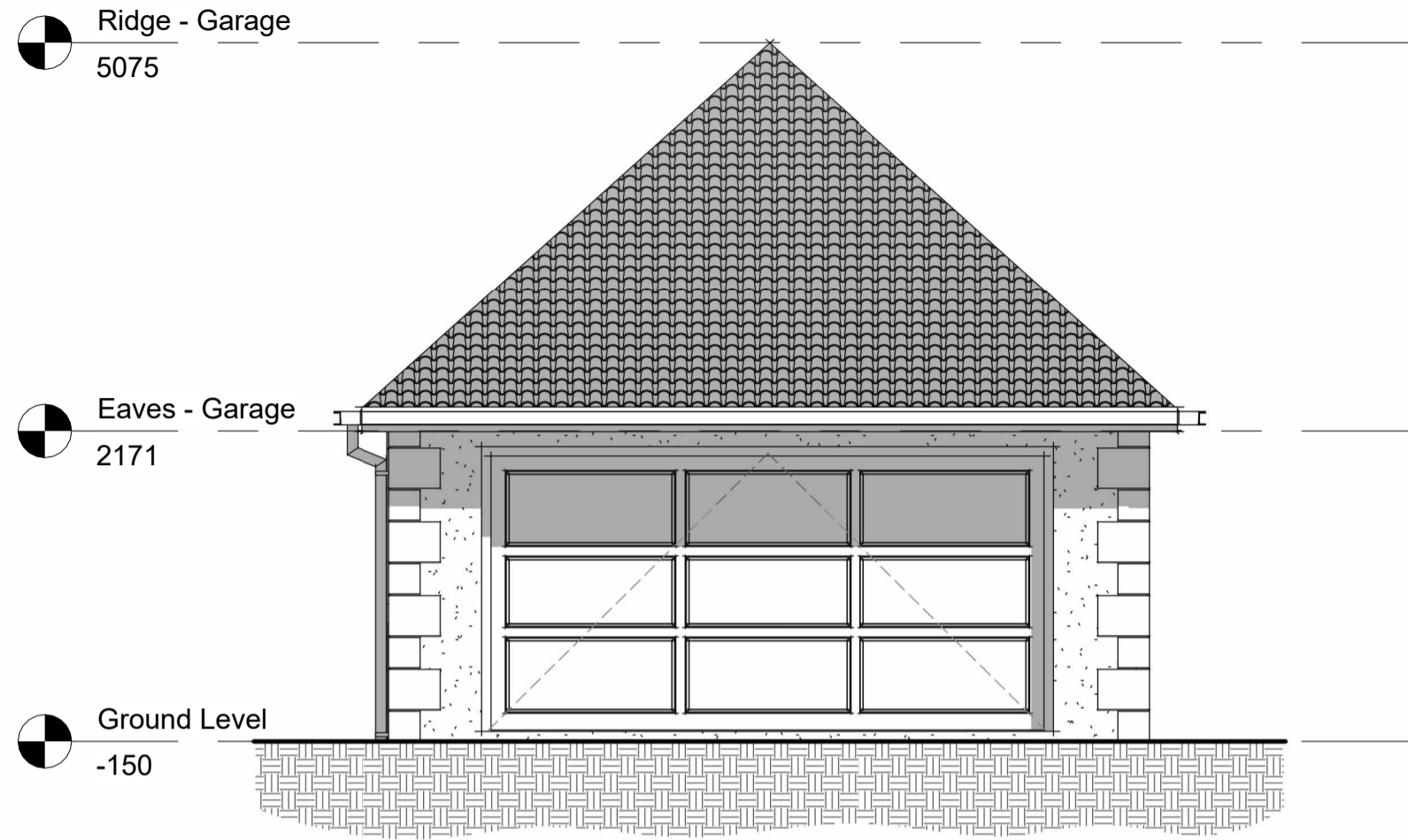
1 FRONT ELEVATION - GARAGE - EXISTING 1 : 50
