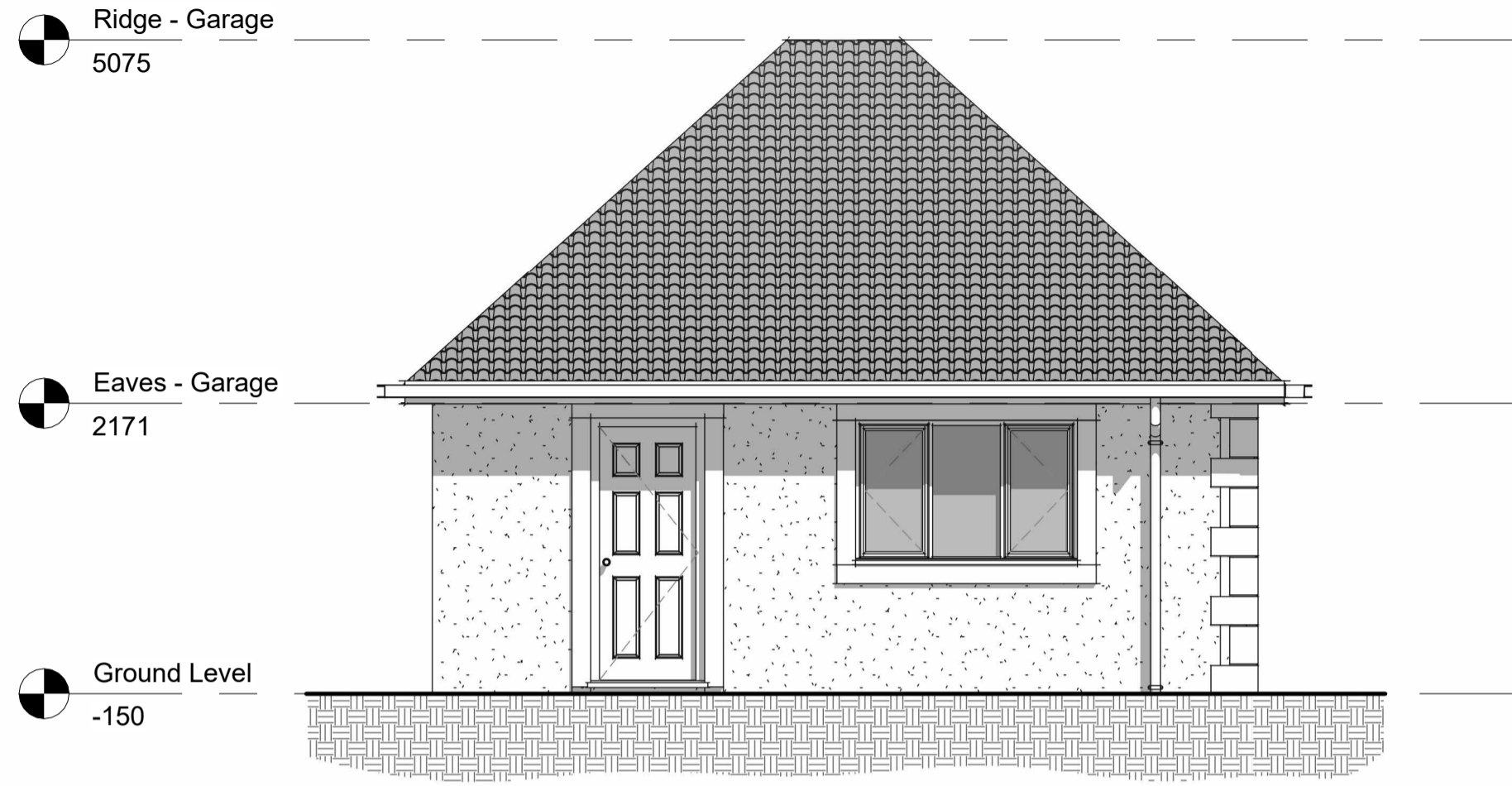
2 SIDE ELEVATION - GARAGE - EXISTING 1 : 50
