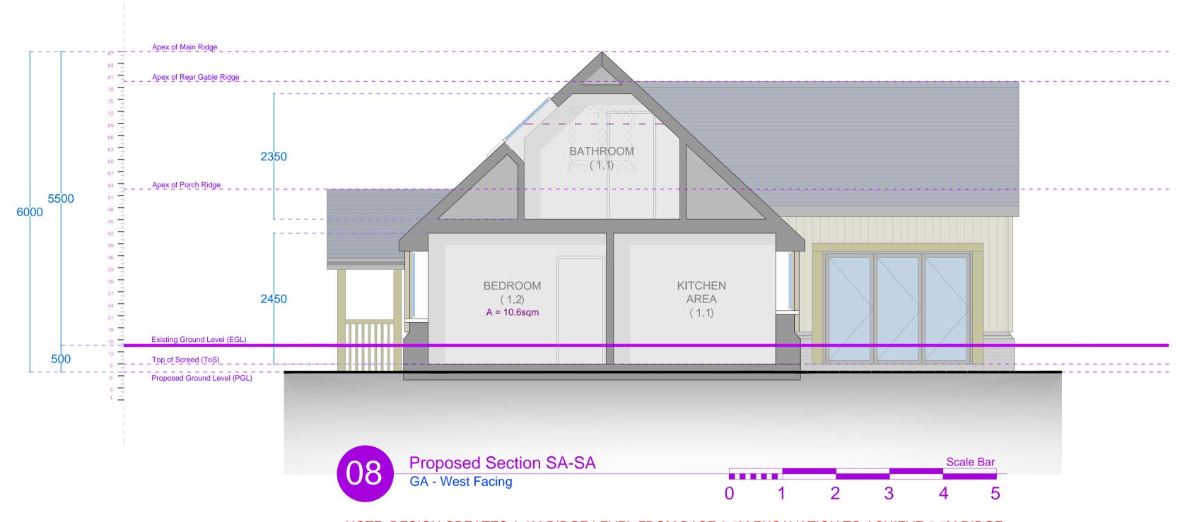
NOTE: DESIGN CREATES A 6M RIDGE LEVEL FROM BASE 0.5M EXCAVATION TO ACHIEVE 5.5M RIDGE TO EXISTING GRD LEVEL WHICH IS ONLY 0.5M HIGHER THAN EXTANT APPROVAL
