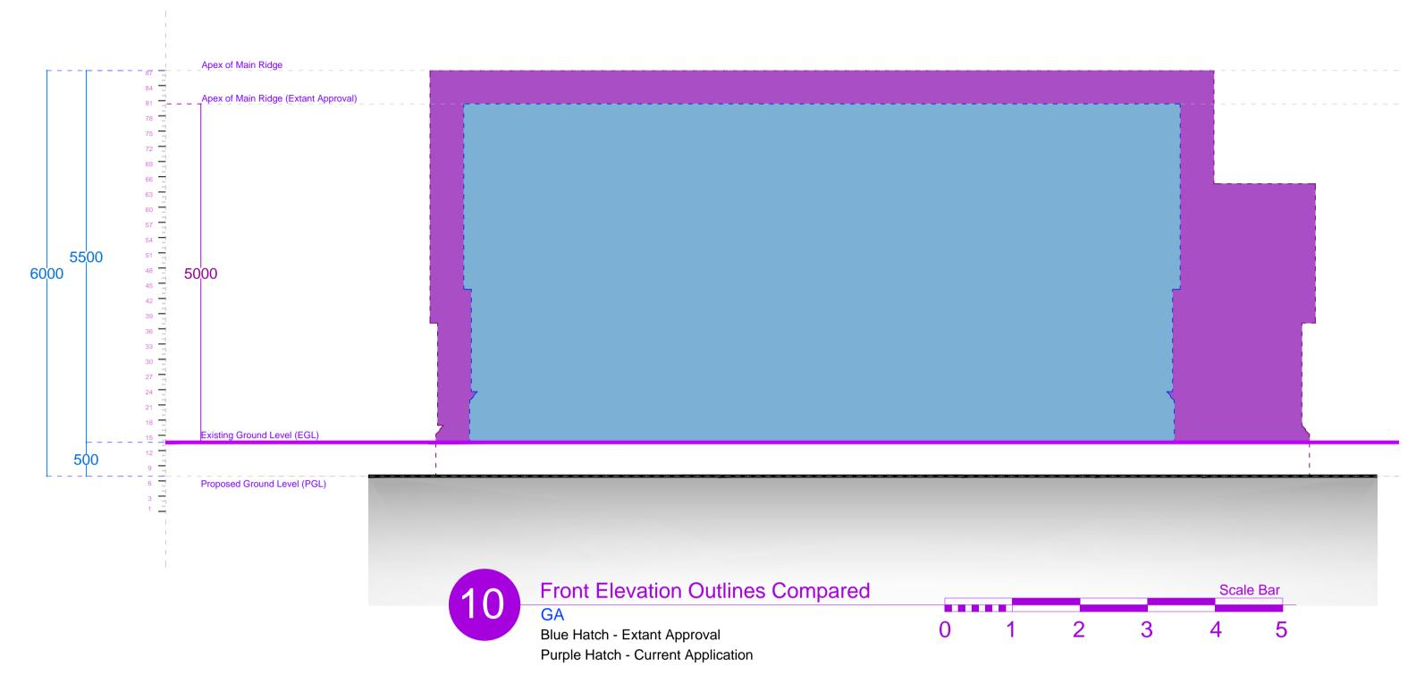
NOTE: DESIGN CREATES A 6M RIDGE LEVEL FROM BASE 0.5M EXCAVATION TO ACHIEVE 5.5M RIDGE TO EXISTING GRD LEVEL WHICH IS ONLY 0.5M HIGHER THAN EXTANT APPROVAL
