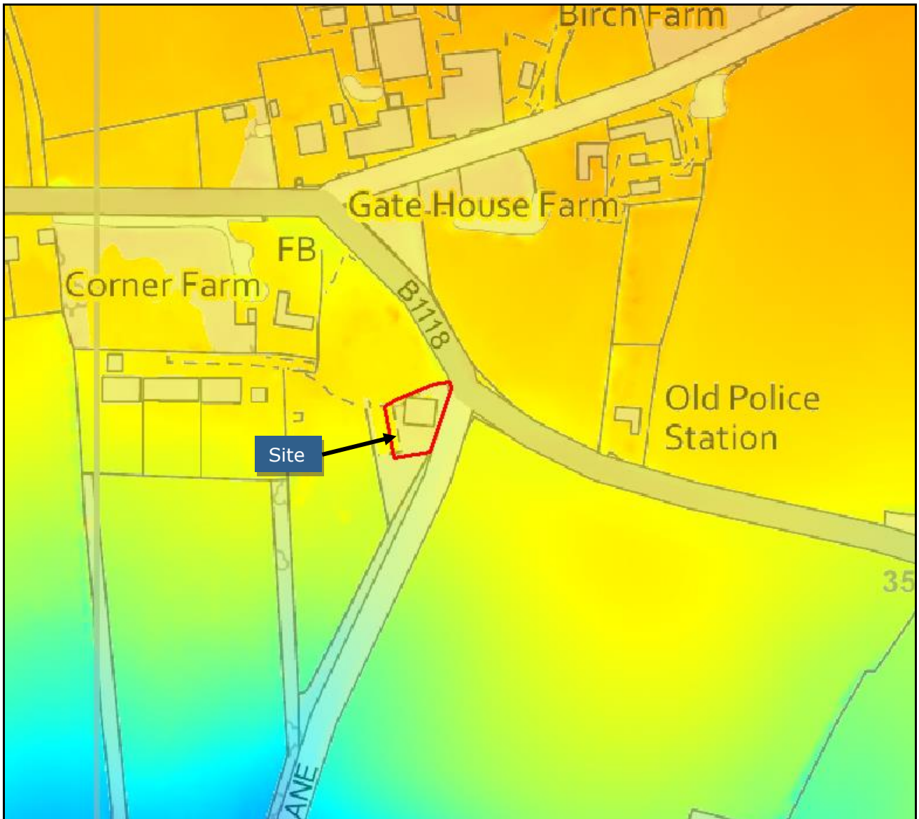
Figure 2: Filtered LIDAR survey data at 1m resolution where higher ground is denoted by red and orange colours and lower ground is denoted by blue colours
