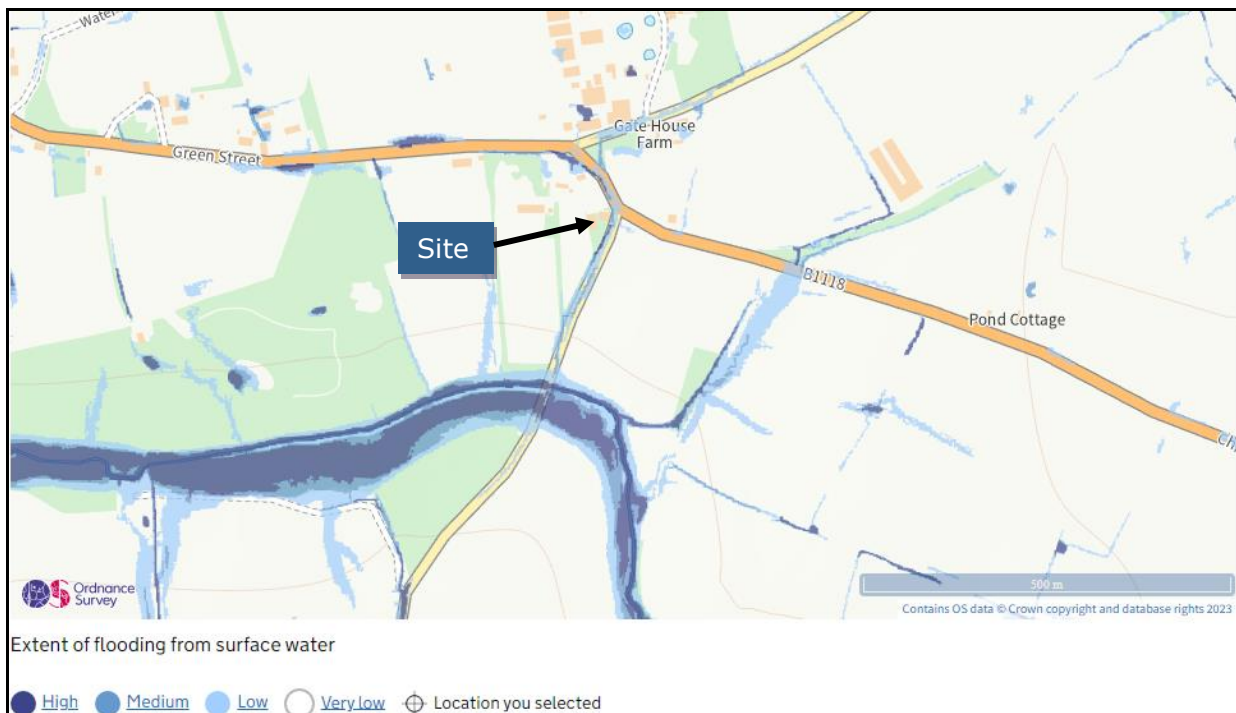
Figure 4: Environment Agency Surface Water Flooding Map (Source: Environment Agency, 2023)
