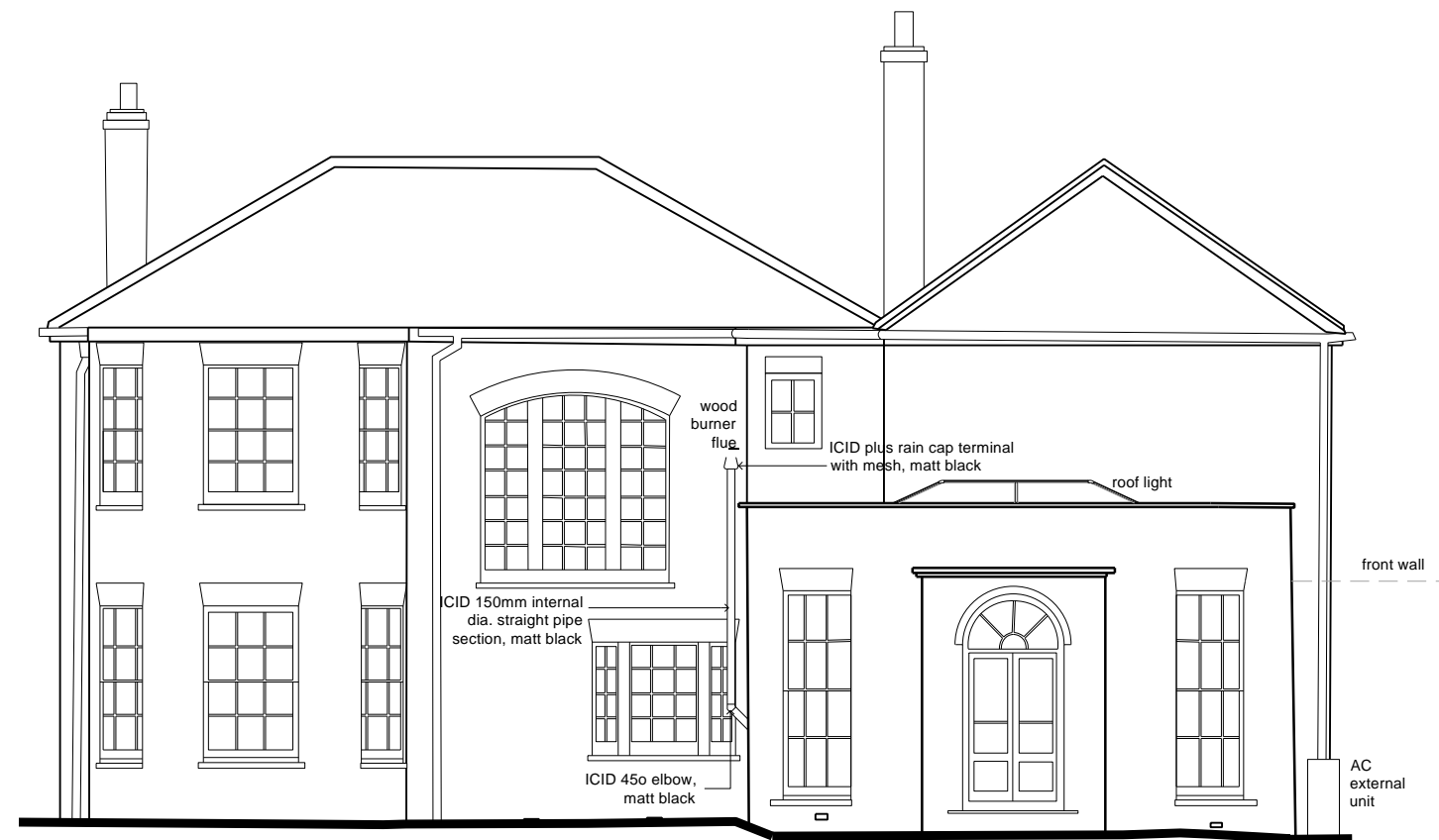
west (side) elevation main dwelling
