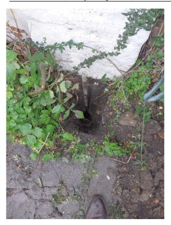
The trial was extended and at 800mm the ground changed to a grey mottled clay again.
