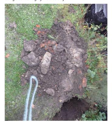
A Mackintosh Probe (a cone penetrometer) gave a result of 9 blows for a 75mm penetration of the ground beneath the foundation which is a soft soil of low bearing capacity.
