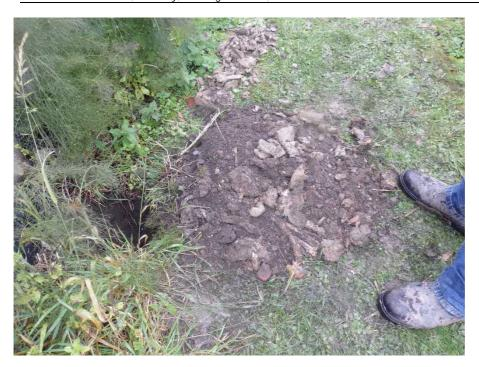
A Mackintosh Probe (a cone penetrometer) gave a result of 10 blows for a 75mm penetration of the ground beneath the foundation which is a soft soil of low bearing capacity.
