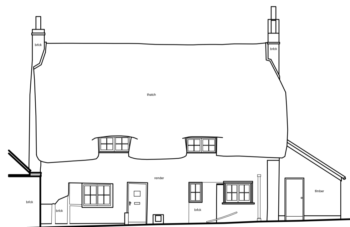
PROPOSED EAST ELEVATION SCALE 1:100 @ A1
