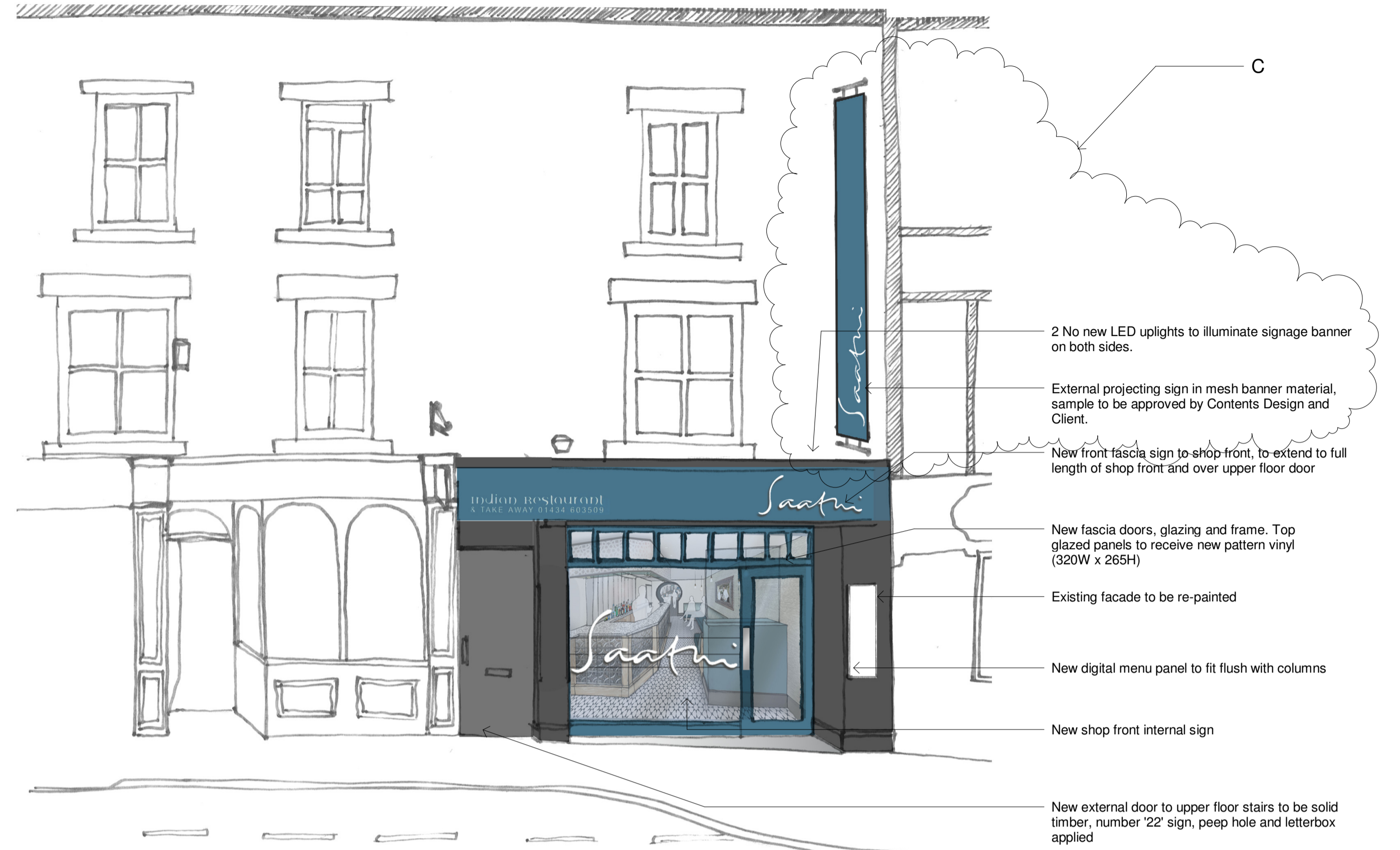
Elevation A - External Elevation Shopfront 1:20
