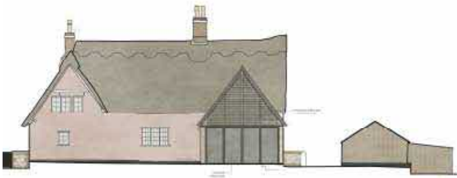
Fig. 2.4.1 Proposed South elevation showing the extensions subservient scale and stepping down in relation to the existing farmhouse
