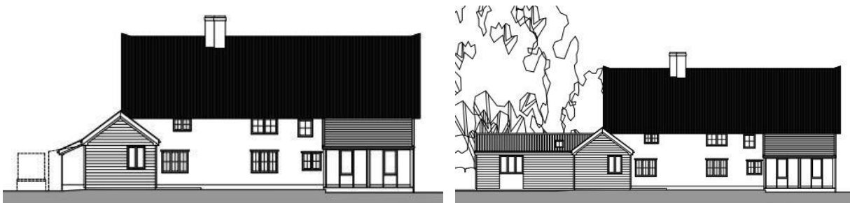
Left: Existing SW elevation, scale 1 : 100 (Nick Barber Architects drawing 1801 10); Right: Proposed SW elevation, scale 1 : 100 (Nick Barber Architects drawing 1801 40)
