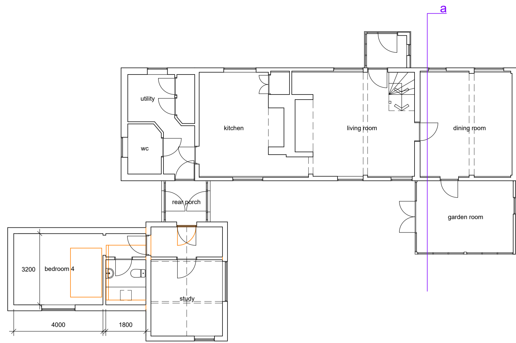
ground floor plan demolitions indicated in orange
