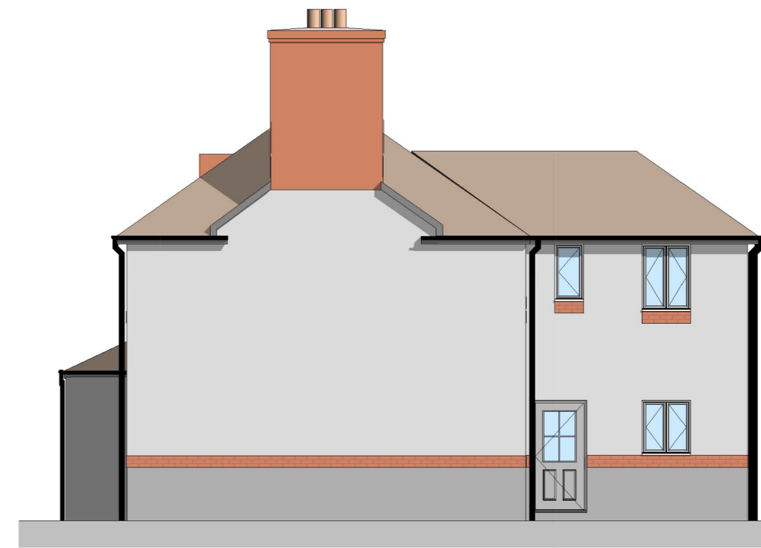
Right Side Elevation Type 1 1 : 100
