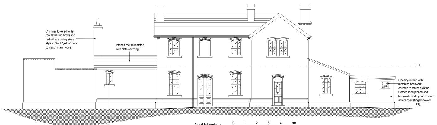
New timber fixed pane window in original openings West Elevation
