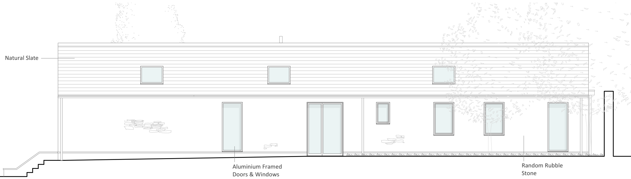
DUNANT HOUSE EAST ELEVATION
