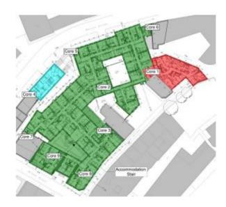
There 9 evacuation routes within the Everards Development each serving multiple floors. They are indicated on the map "Core". The main core, servicing the Commercial Printworks area is Core 6.
