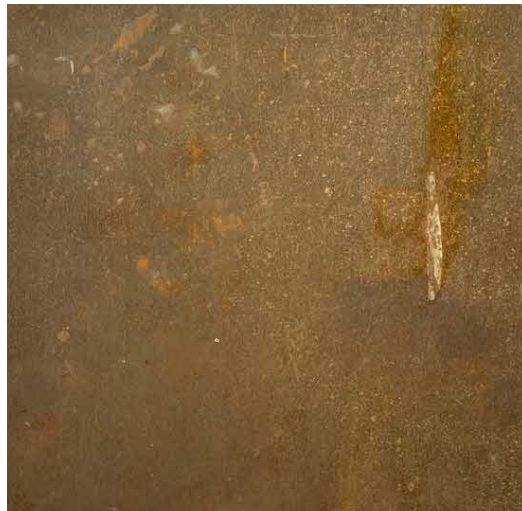
Image 1 – example of copper cladding following a short weathering period
