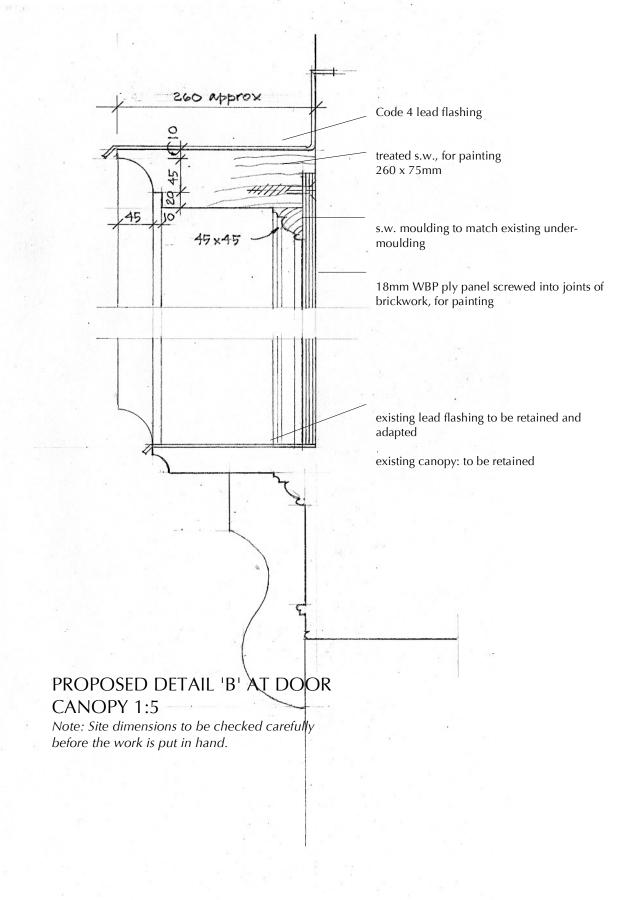
REVISION A - 11.10.23 - Lead flashing added; dimension of cornice.
