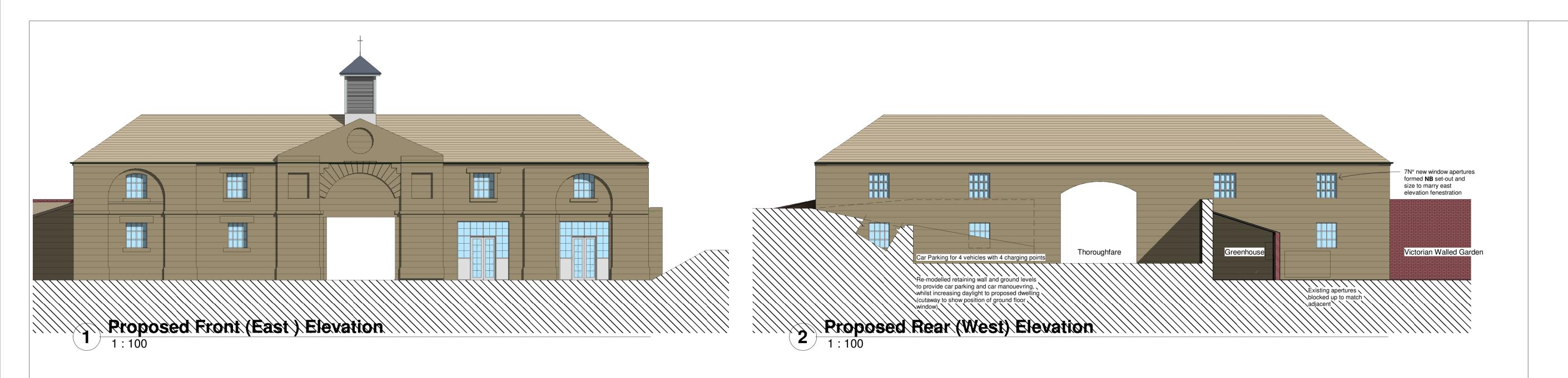
Existing infill removed from former aperture and replaced with stone to match adjacent
